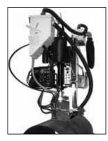
The **CWP-18 Programmable Circle Welder** is designed for single or multi-pass welding of couplings or nozzles into vessels or domed heads utilizing Sub-Arc, MIG or Flux Core process with gas shielding. The CWP-18 mounts on a 3 jaw chuck for welding diameters of 10-50" (254-1270 mm) O.D.
