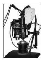
The **CWP-11 Programmable Circle Welder** is designed for welding of nozzles into vessels utilizing Sub-Arc, MIG or Flux Cored Process. The CWP-11 mounts on a 3-Jaw Chuck for welding diameter 6-50" (152-1270 mm) O.D.
