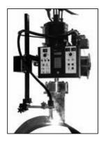
The **CWP-5 Programmable Circle Welder** is designed for single or multi-pass welding of couplings or nozzles utilizing MIG or Flux Core process capable of welding 1-12" (25-305 mm) diameters.
