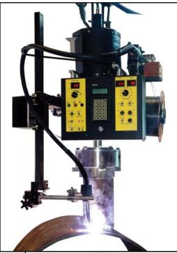
The **CWP-5 Programmable Circle Welder (CWP-1500)** is designed for single or multi-pass welding of couplings or nozzles utilizing MIG or Flux Core process capable of welding 1-12" (25-305 mm) diameters. This machine uses a microprocessor to control the rise and fall through encoder position.
