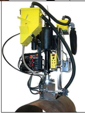
The **CWP-18 Programmable Circle Welder (CWP-1800-SA)** is designed for single or multi-pass welding of couplings or nozzles into vessels or domed heads utilizing Sub-Arc, MIG or Flux Core process with gas shielding. The CWP-18 mounts on a 3 jaw chuck for welding diameters of 10-50" (254-1270 mm) O.D. This machine uses a microprocessor to control the rise and fall through encoder positioning. Photo shown with optional Flux Recovery System installed.
