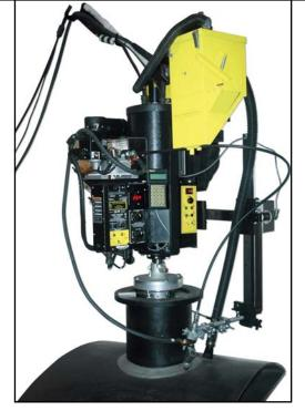
The **CWP-11 Programmable Circle Welder** (**CWP-1100**) is designed for welding of nozzles into vessels utilizing Sub-Arc, MIG or Flux Cored Process. The CWP-11 mounts on a 3-Jaw Chuck for welding diameter 6-50" (152-1270 mm) O.D. The machine uses a microprocessor to control the rise and fall through encoder positioning. Photo shown with optional Flux Recovery System installed.
