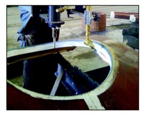
For straight or beveled flame cut holes on domed heads, vessels and large diameter pipe, without wrap-up of power cable or gas hoses (CBP-3000 - 120/50-60/1). 220 Volt also available (CBP-3002).
